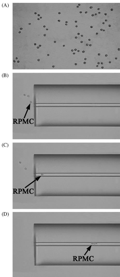
**Fig. 2.** Process of the injection and lysis of single cells. (A) The single RPMCs on the slide under the view of microscope; (B) a mast cell drifting toward the injection end; (C) the whole cell into the separation capillary tip; (D) the mast cell lysed.
