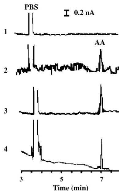
**Fig. 5.** Electropherograms of 1, PBS; 2, the single RPMC (without a holder); 3 and 4, the single RPMCs (with a holder). Other conditions as in Fig. 3.
