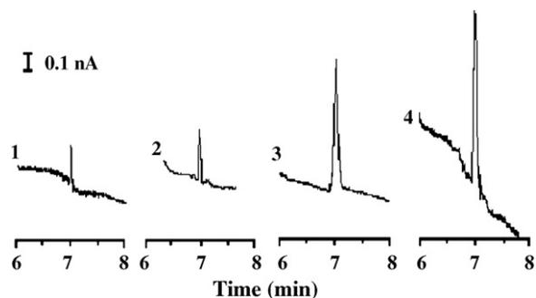
**Fig. 4.** Electropherograms of mast cell extract without and with the standard solution of AA. The added concentration of AA: 1, 0 mol/l; 2,  $6.94 \times 10^{-6}$  mol/l; 3,  $2.50 \times 10^{-5}$  mol/l; 4,  $4.31 \times 10^{-5}$  mol/l. Other conditions as in Fig. 3.
