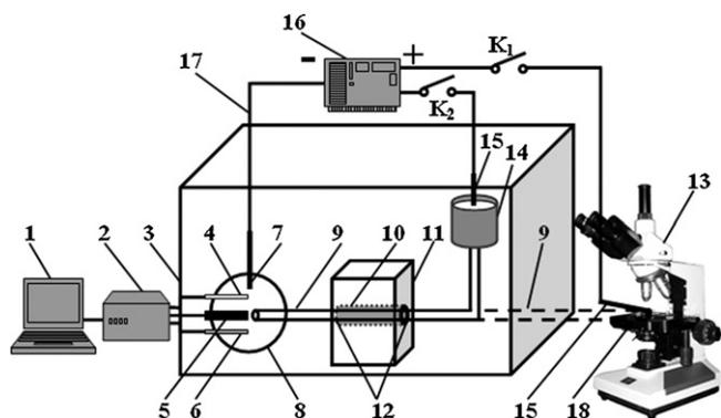
**Fig. 1.** Overview of the CE-ED detection and the single-cell analysis system. 1, computer; 2, electrochemical detector; 3, Faraday cage; 4, reference electrode; 5, working electrode; 6, auxiliary electrode; 7, high-voltage cathode; 8, CE-ED detection cell; 9, capillary; 10, rubber tube; 11, foam holder; 12, silicone glass sealant; 13, inverted microscope; 14, running buffer reservoir; 15, high-voltage anode; 16, high voltage; 17, copper wire; 18, setup of single-cell injection [19].
